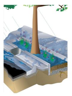
Stormwater tree pits are designed to increase infiltration through inlets and pervious surfaces. Trees transpire water, reducing the amount of water entering constructed runoff management systems.
