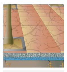
Permeable pavements (surface shown above) increase infiltration, allowing more runoff to be absorbed and available for use by the tree.
