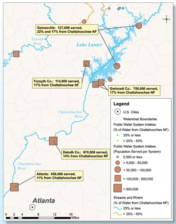
**Figure 9**—Intakes serving the greater Atlanta, GA, area with water from the Chattahoochee National Forest and regulated by the Buford Dam at Lake Lanier.
