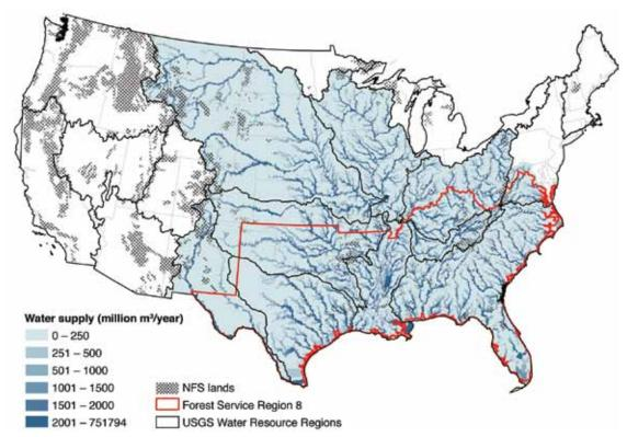
**Figure 4**—Predicted 2001–2010 mean annual water supply in millions of cubic meters per year by 12-digit (sixth level) hydrologic unit code (HUC) watershed for those watersheds supplying water to the South. HUCs are colored by the magnitude of available water supply at the HUC outlet.
