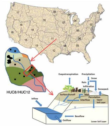
**Figure 2**—Schematic diagram illustrating the hydrological processes simulated by the Water Supply Stress Index Model (WaSSI). WaSSI uses national scale databases to predict water supply over the conterminous U.S. at the HUC12 scale.
