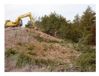
Grinders can be used to reduce brush piles along the firebreak. Grinders can reduce large trees into smaller piles of chips, which are much safer than large piles of whole trees.
