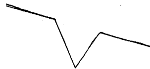
Figure 2-3. Small channel on sloping road
