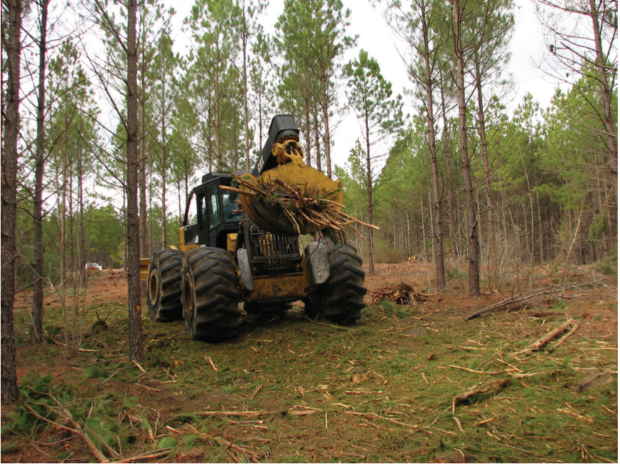
Figure 22. Scattering Logging Slash or Other Mulch Material on Skid Trail.
